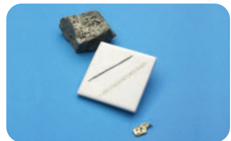
Figure 5 During the gold rush, prospectors used streak to test if they had found real gold.
